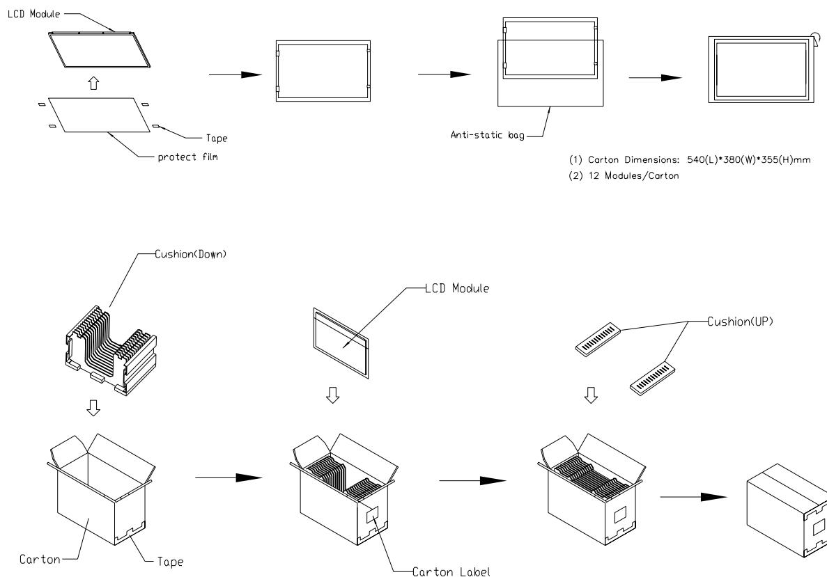
**Figure. 8-1 Packing method**
