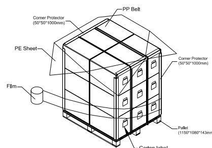
**Figure. 8-2 Packing method**
